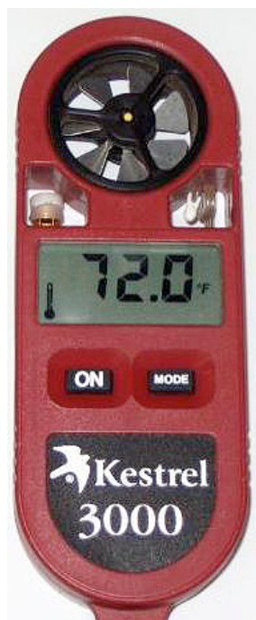
Figure 2. Examples of wind meters used for determining wind speed, temperature, and humidity.
